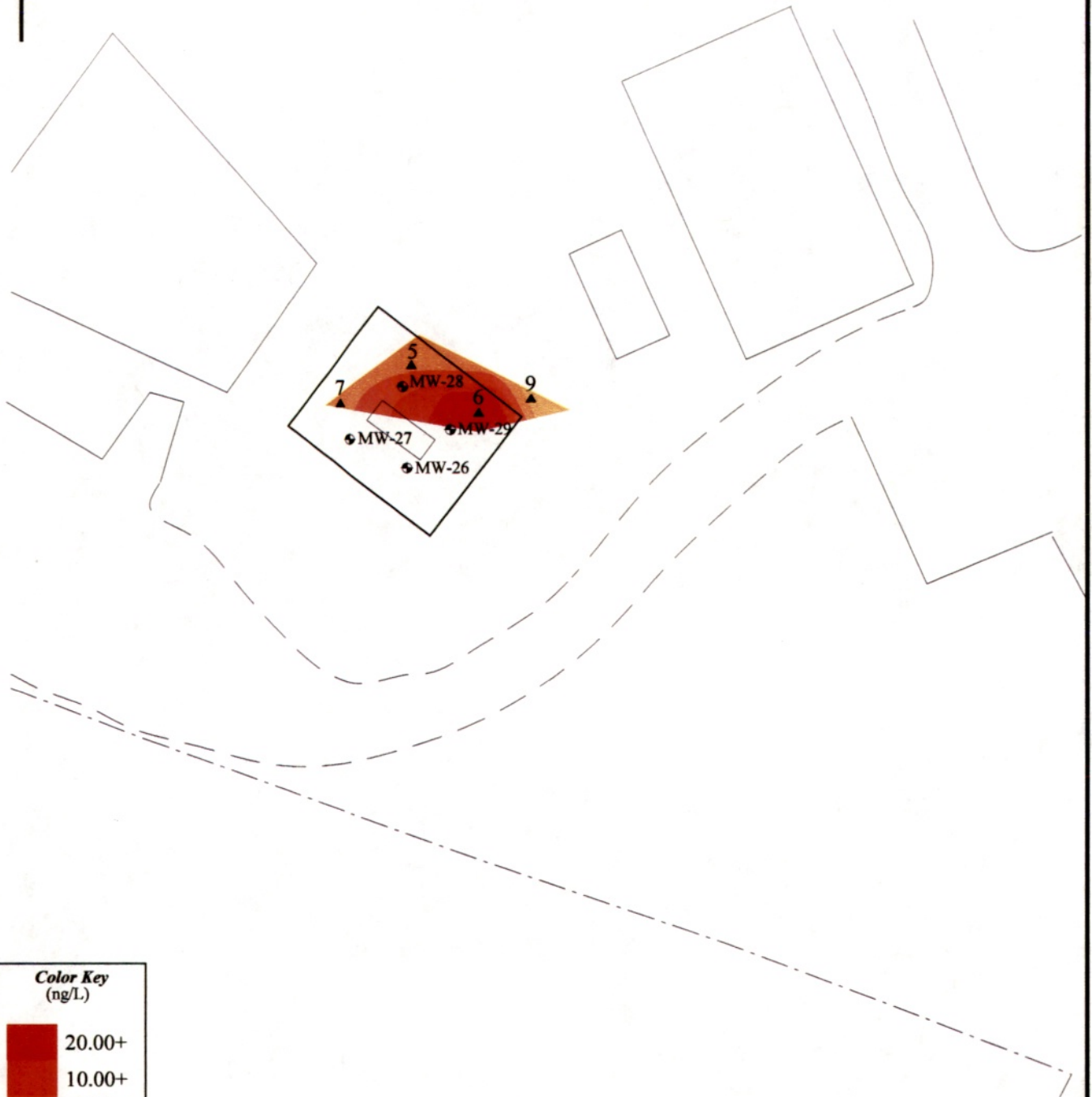
Figure 4 Trichloroethene Isopleths Pit CW-1 Fort Monmouth, NJ EMFLUX Sample Point Fence Road/Trails (unpaved) NOTES: The reported soil-gas concentration quantitation level for Trichloroethene is 0.09 ng/L. Sample point 8 was designated as the trip blank.
