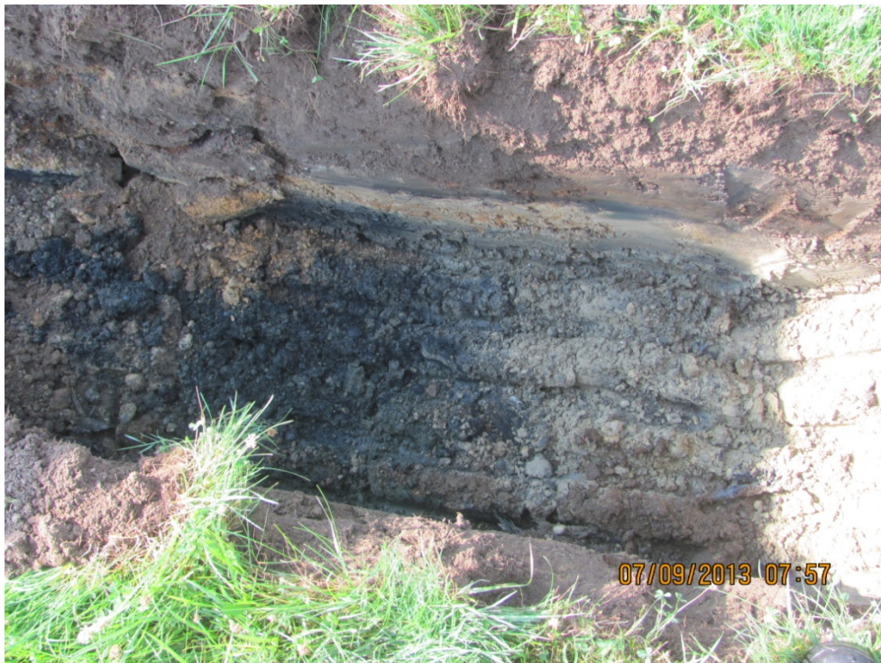
2. IMG002 Test Pit FFSGC-C. Field notes indicated “Burnt wood, fill dirt with black organic material, glauconitic clay, no odor + terracotta pipe section.”
