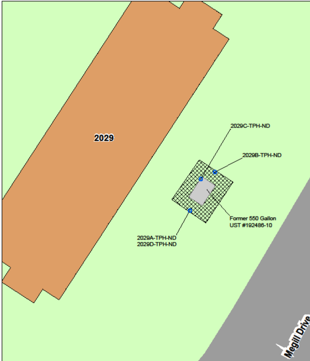
Figure 3 Soil Sampling Location Map Building 2029, Charles Wood Area Fort Monmouth, NJ Date: 1/2011 UST Registration # 192486-10 UST Discharge # NA
