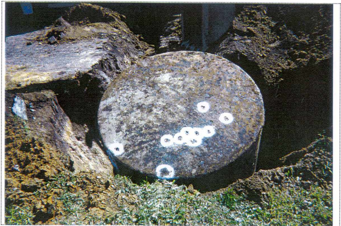
PHOTO 2: View of the eastern end of UST-9031 showing holes (circled with white paint) (looking west).
